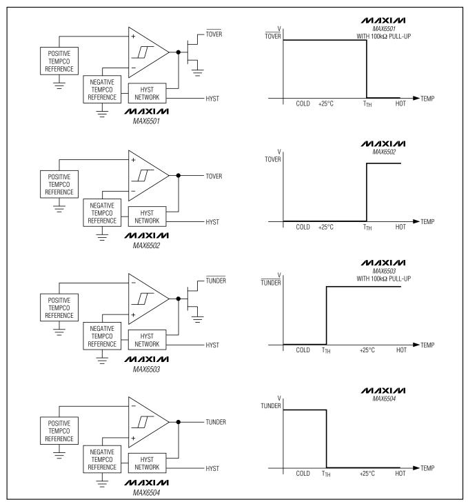
Figure 1. Block and Functional Diagrams
