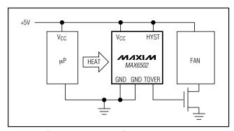
Figure 3. Overtemperature Fan Control
