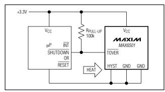
Figure 2. Microprocessor Alarm/Reset
