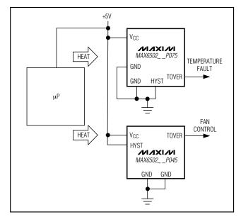
Figure 5. Low-Power, High-Reliability, Fail-Safe Temperature Monitor
