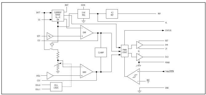
Figure 2. Functional Diagram
