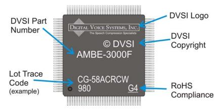
Figure 5 AMBE-3000F<sup>™</sup> Vocoder Chip LQFP Markings
