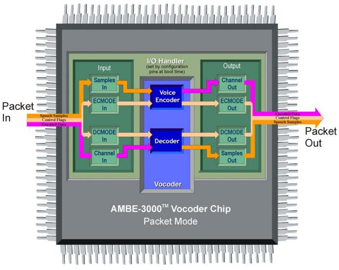
Figure 28 Interface Block Diagram Packet Mode
