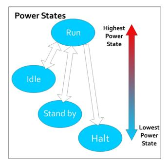
Figure 14 AMBE-3000F<sup>™</sup> Vocoder Chip Power States
