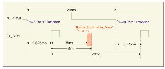
Figure 23 TX\_RDY with Skew Control On
