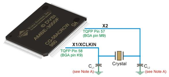
Figure 8 X1/XCLKIN and X2 with Crystal Oscillator
