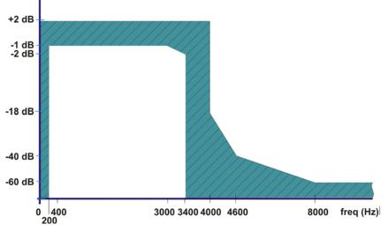
Figure 38 Front End Output Filter Mask
