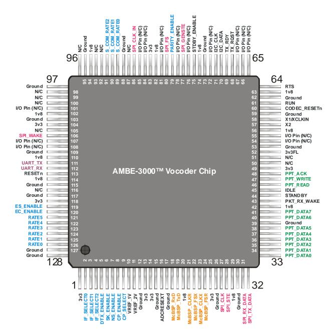
Figure 3 AMBE-3000F™ Vocoder Chip Pins for LQFP Package
