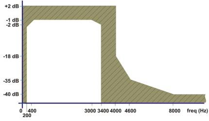
Figure 37 Front End Input Filter Mask
