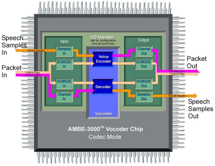
Figure 27 Interface BLOCK Diagram Codec Mode
