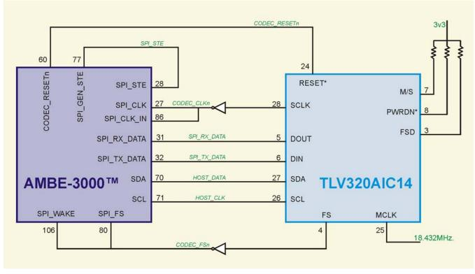
Figure 39 AMBE-3000F<sup>™</sup> Vocoder Chip and TLV320AIC14 Interface Block Diagram
