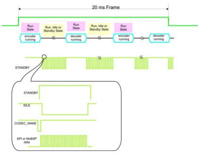
Figure 15 Power Mode States Basic Timing
