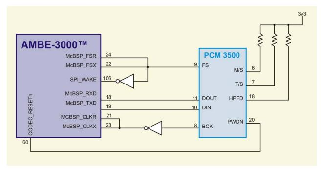
Figure 40 AMBE-3000F<sup>™</sup> Vocoder Chip and PCM3500 Interface Block Diagram
