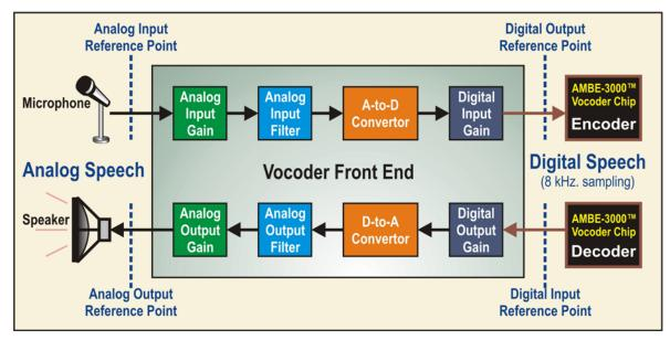
Figure 36 Vocoder Front End
