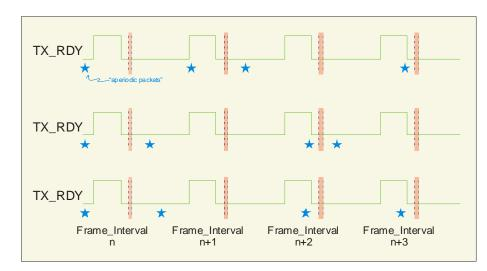
The following figure shows some examples of packet timing that are aperiodic
