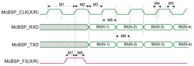
Figure 32 Timing of McBSP When Selected as Codec Interface
