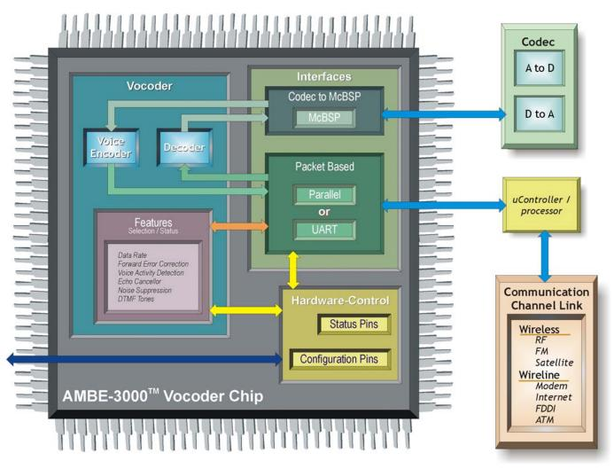
Figure 21 Codec Mode (McBSP Interface)
