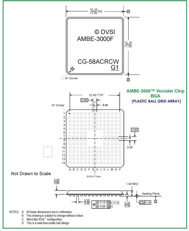
Figure 2 BGA Mechanical Details
