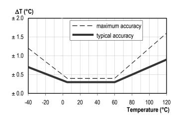
Figure 3 Typical and maximal temperature accuracy tolerance
