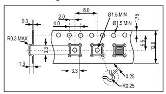
**Figure 14** Sketch of packaging tape and sensor orientation. Header tape is to the right and trailer tape to the left on this sketch.
