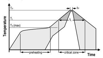
**Figure 7** Soldering profile according to JEDEC standard.  $T_P \le 260^{\circ}\text{C}$  and  $t_P \le 30\text{sec}$  for Pb-free assembly.  $T_L \le 220^{\circ}\text{C}$  and  $t_L \le 150\text{sec}$ . Ramp-up/down speeds shall be  $\le 5^{\circ}\text{C/sec}$ .
