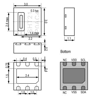
**Figure 1:** Drawing of SHT21P sensor package, dimensions are given in mm (1mm = 0.039inch), tolerances are  $\pm 0.1$ mm. The die pad (center pad) is internally connected to VSS. The NC pads must be left floating. Numbering of E/O pads starts at lower right corner (indicated by notch in die pad) and goes clockwise (compare Table 2).
