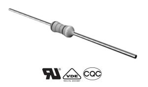
A metal glazed film is deposited on a high grade ceramic body. After a helical groove has been cut in the resistive layer, tinned electrolytic copper wires are welded to the end-caps. The resistors are coated with a light blue lacquer which provides electrical, mechanical, and climatic protection.
