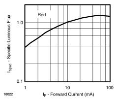
Figure 11. Specific Luminous Flux vs. Forward Current
