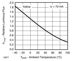
Figure 14. Rel. Luminous Flux vs. Ambient Temperature
