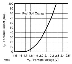
Figure 7. Forward Current vs. Forward Voltage
