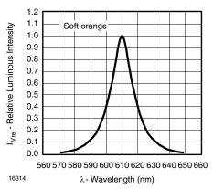
Figure 6. Relative Intensity vs. Wavelength
