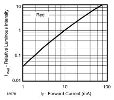
Figure 9. Relative Luminous Flux vs. Forward Current
