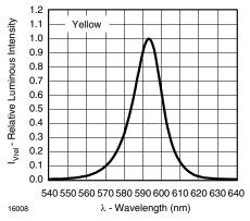
Figure 5. Relative Intensity vs. Wavelength
