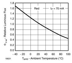
Figure 13. Rel. Luminous Flux vs. Ambient Temperature
