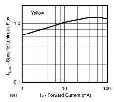
Figure 12. Specific Luminous Flux vs. Forward Current
