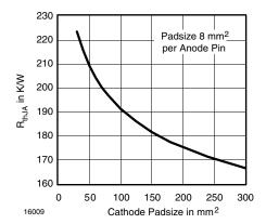
Figure 15. Thermal Resistance Junction Ambient vs.
