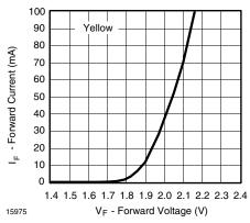
Figure 8. Forward Current vs. Forward Voltage
