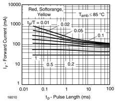
Figure 2. Forward Current vs. Pulse Length
