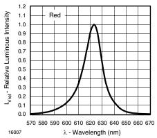
Figure 4. Relative Intensity vs. Wavelength
