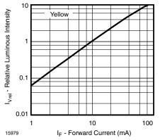
Figure 10. Relative Luminous Flux vs. Forward Current
