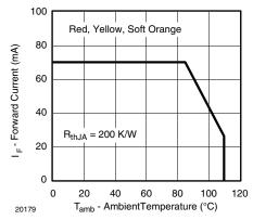
Figure 1. Forward Current vs. Ambient Temperature
