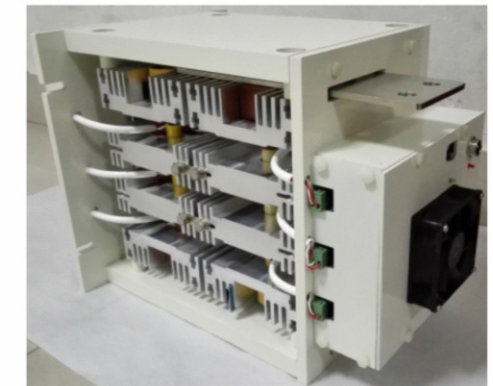
Fig.2 风冷脉冲功率组件 Fig.2 Air-cooling Pulsed Power Assemblies
